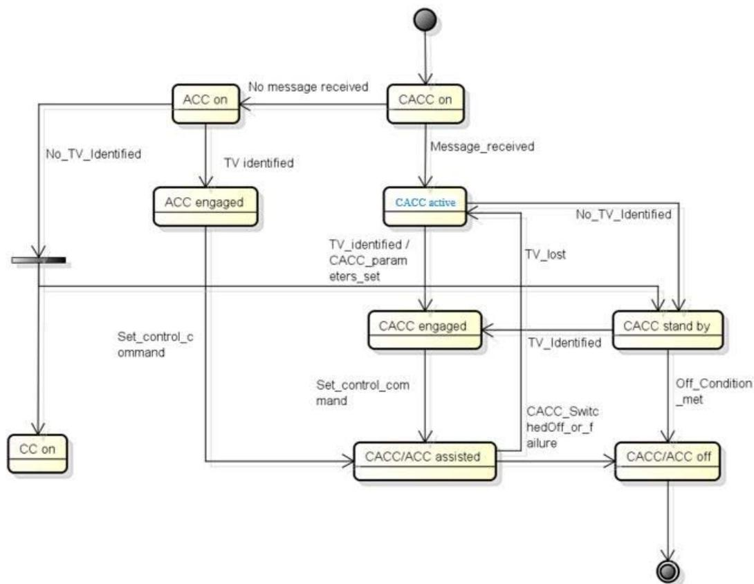
Figure B.1: CACC application state machine diagram
