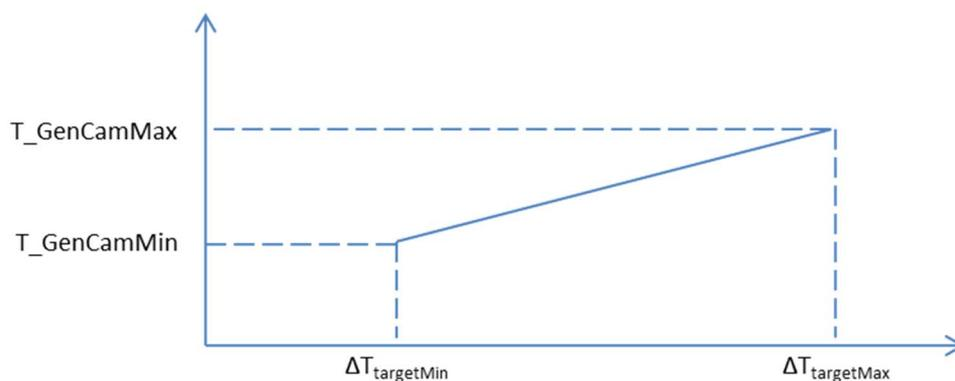
**Figure 13:  $T\_GenCam$  value setting rule for CACC**
