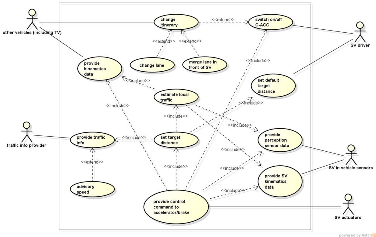
Figure 5: Use case diagram: follow TV with dynamically configured distance
