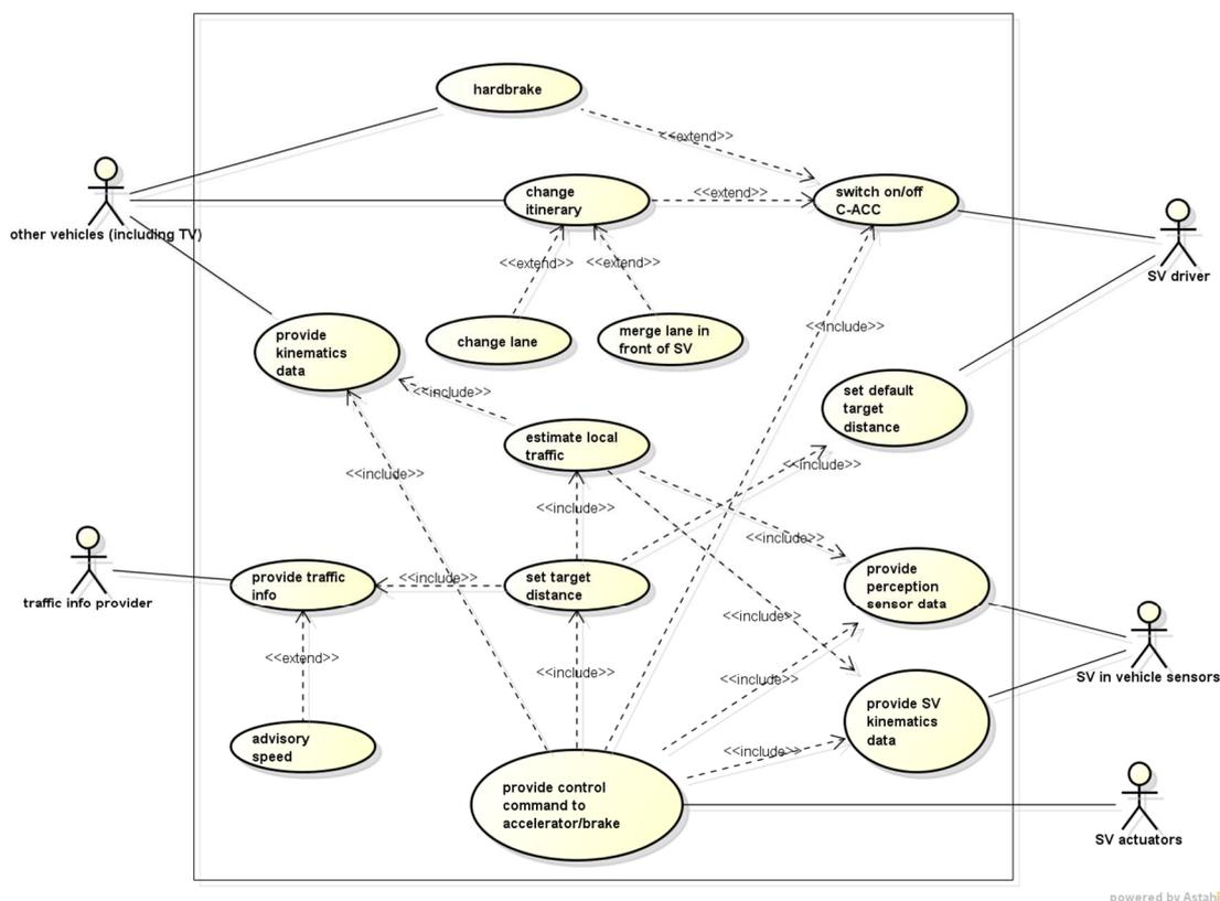
Figure 3: Use case diagram: follow TV with configured time gap
