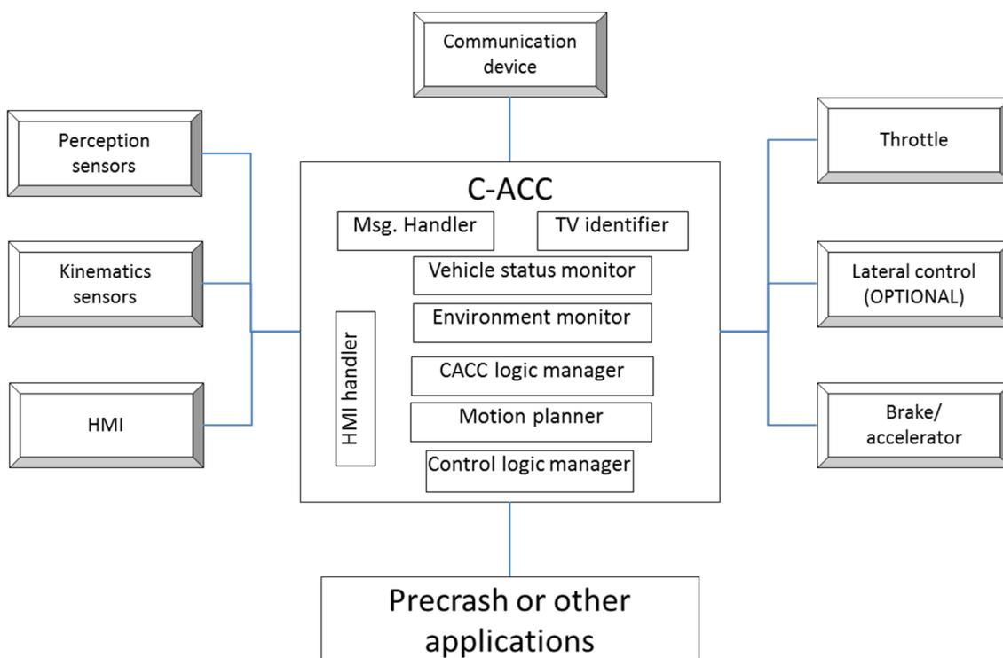
Figure 10: CACC Functional architecture
