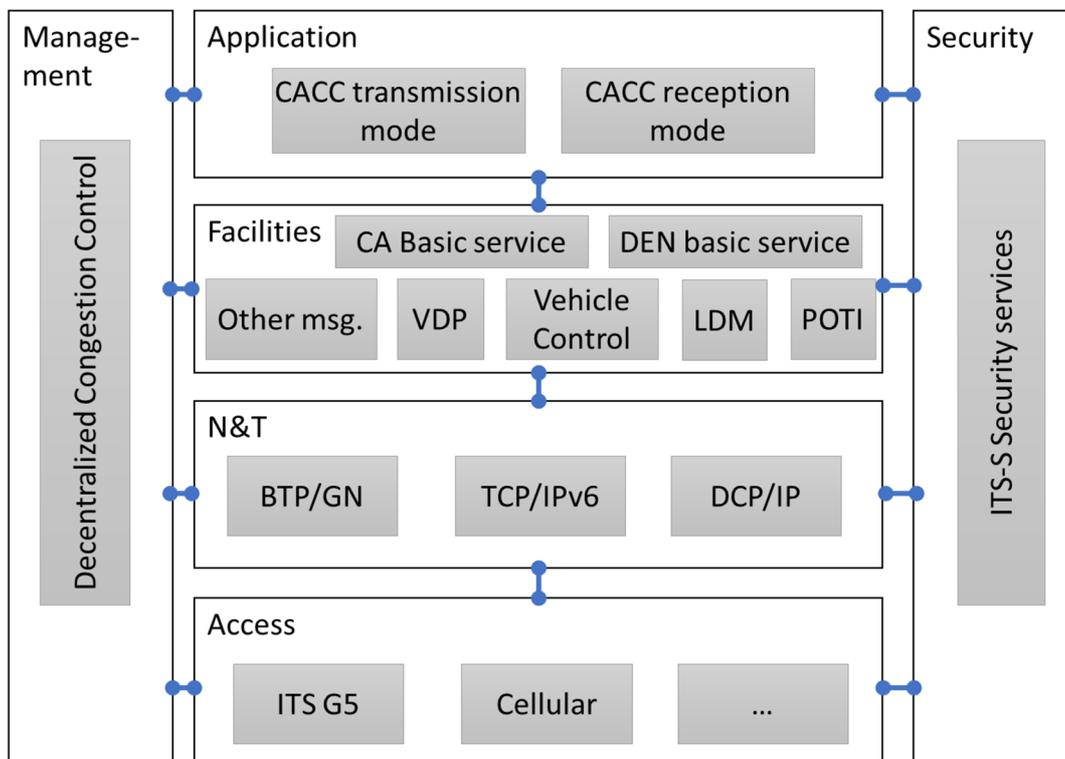
Figure 12: CACC communication architecture
