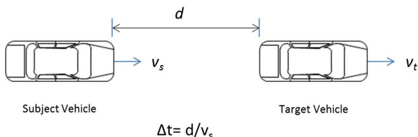
**Figure 2: CACC target time gap**
